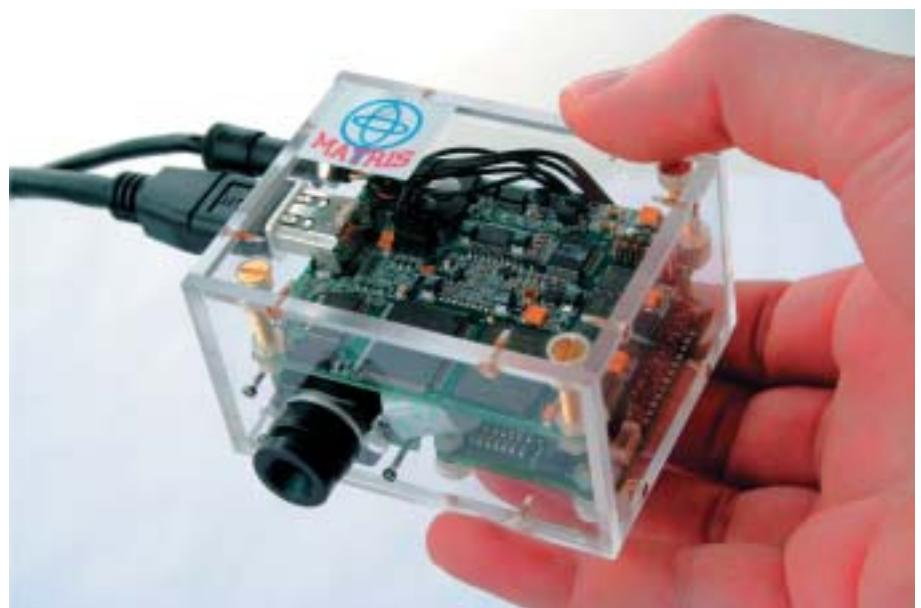
Figure 1: MATRIS – integrated sensor unit combining inertial sensors and video camera.
