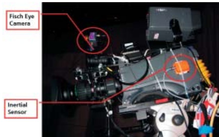
Figure 2: MATRIS technology used for tracking in TV-production.
