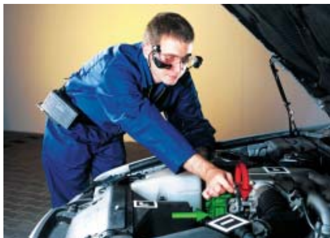
Figure 1: The virtual animation shows the step-by-step repairation procedure
