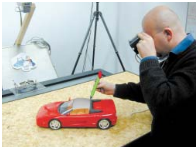
Figure 1: Free from surface sketching in Augmented Reality
