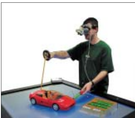
Figure 3: Virtual 3D taping on a physical model in AR
